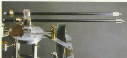
Apply vibrations to the base of a conventional design tonearm; the arm will vibrate together with the base. But the D-O-B tonearm, subjected to the same test, does not vibrate.
